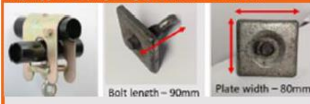
The fitting (photo 2&3) weights 700g & fell 7.25m onto access road below
