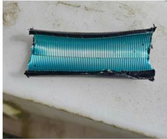
Outer Armoured Cable that caused the injury
