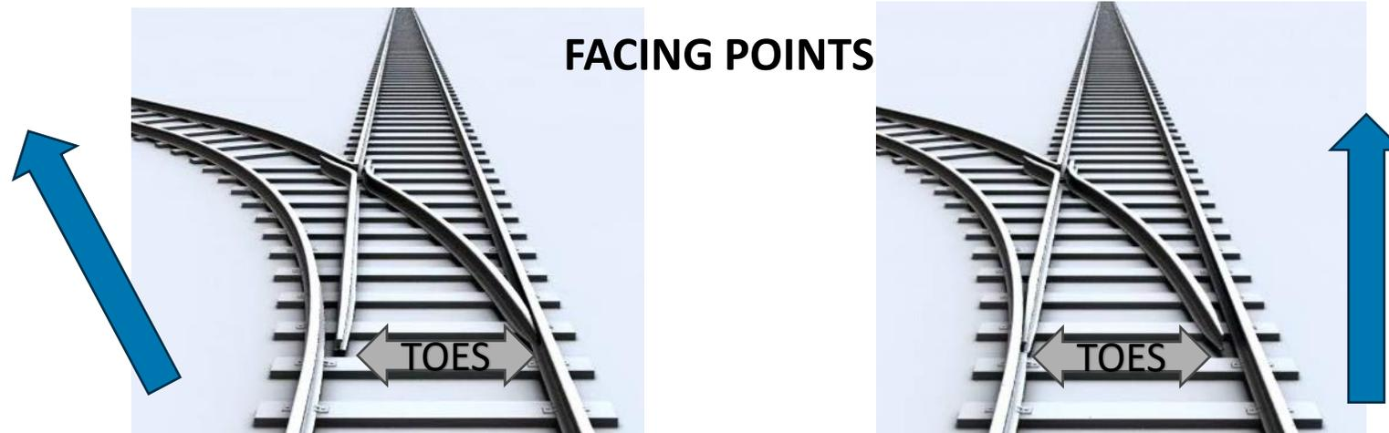
If, as you are approaching the switch, you can see the rail toe ends like the images above then the points are classed as “facing”. The points on the left would route a train to the left, while the points on the right would route a train to carry on straight ahead, it does not matter which direction the route is set to, the important thing to understand is that the points are classed as facing because you are approaching them from the toe ends.
