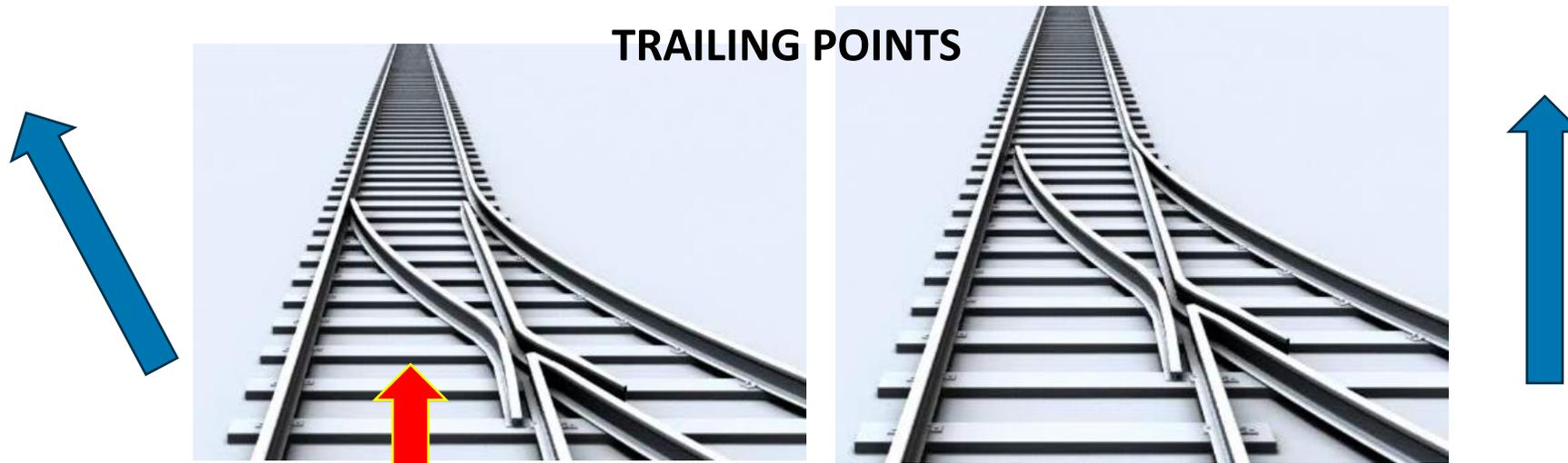
Both of the points in the images above are defined as Trailing, because you cannot see the ends of the point toes, and you would move over the crossing section of the points before the Switch rail section. If you look carefully at the switch rails in these two images you can see that the route setting is different in both of the images.
