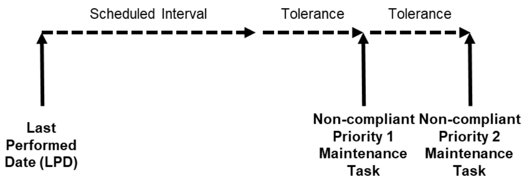
Figure 3 – Missed maintenance beyond tolerance
