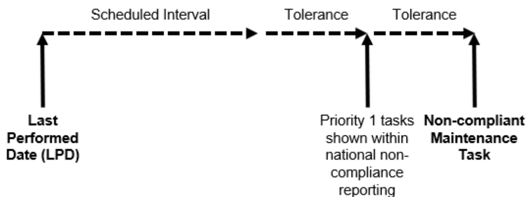
Figure 3 – Missed maintenance beyond tolerance
