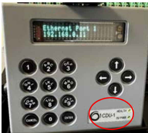
Figure 3 – Health and Power LEDs on CDU-1
