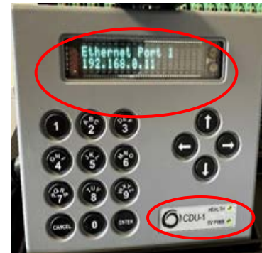
Figure 3 – Health and Power LEDs on CDU-1
