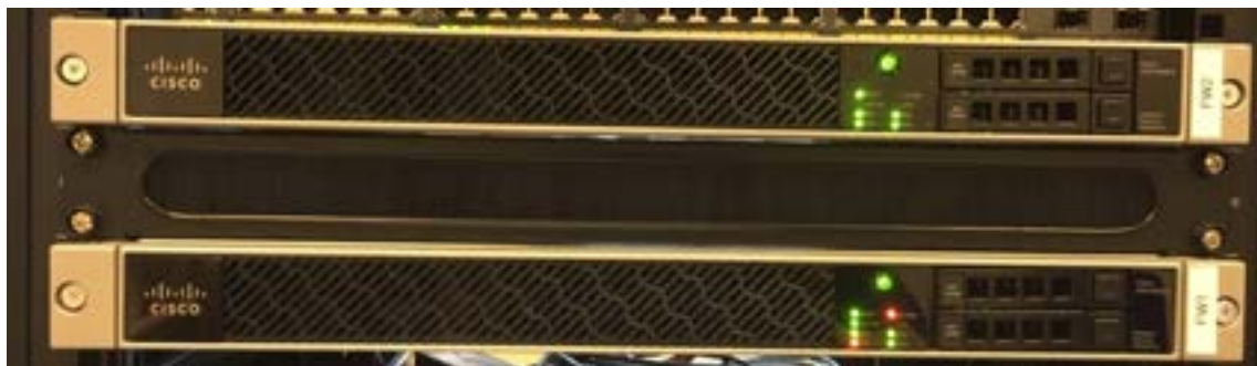
Figure 13 - Status Lights on Front of Firewall
