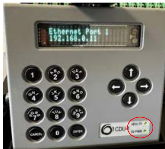
Figure 4 – Health LEDs on CDU-1
