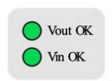
Figure 1 - PS module operational mode indications
