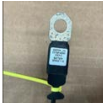
Figure 7 – Thermal Probe unit secured
