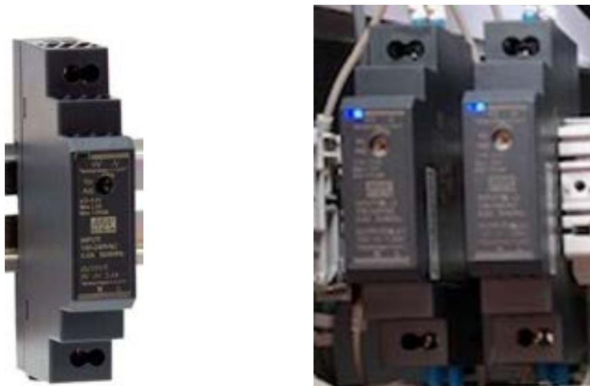
Figure 1 – Meanwell PSU (Unpowered / Powered)
