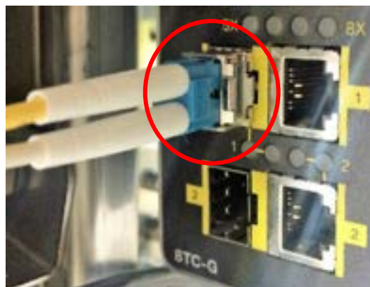
Figure 2 - CISCO Transceiver Module located in switch
