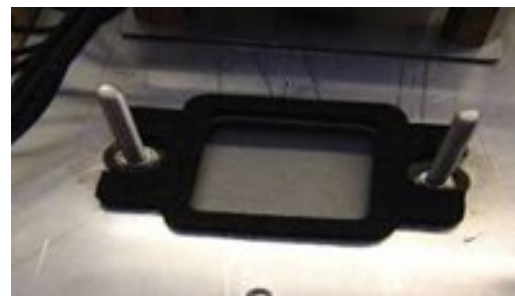
Figure 7 – New gasket fitted
