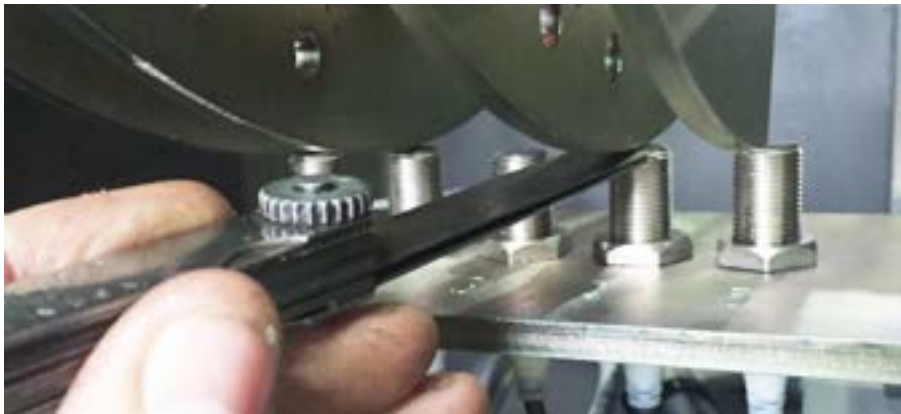
Figure 2 - Position of gauges with the 1.5 mm gauge (Inserted)
