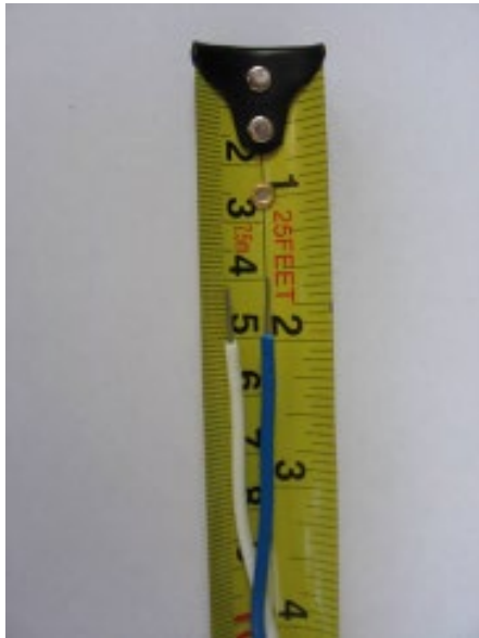
Figure 1 – Cables Stripped to a minimum of 8mm
