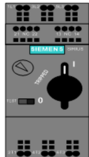
Figure 1 - Incoming supply switch
