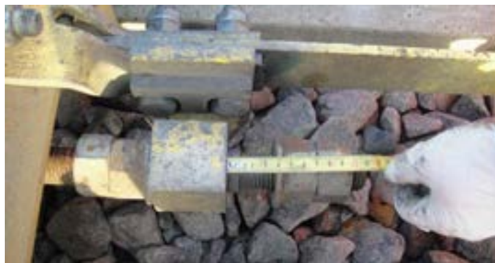
Figure 1 – Photo of Escapement Measurement
